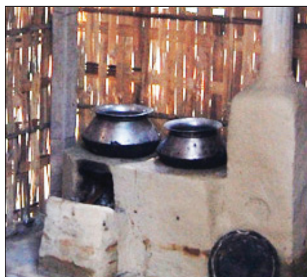
A demonstration model of the 100-Dollar Kitchen with improved cook stove in Shahjadpur sub-district.
