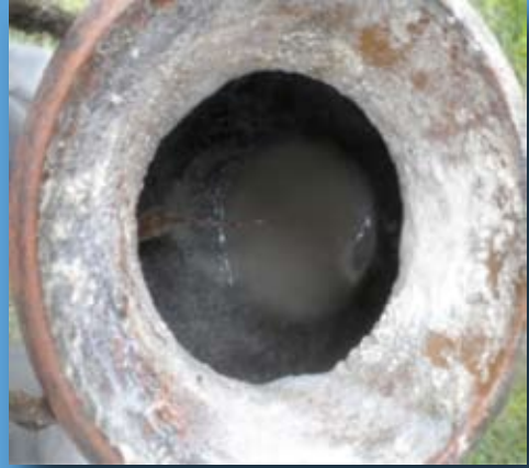
Photo 2: Sediment at the bottom of the pot
