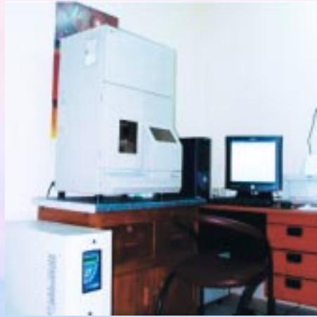
ABI Prism 310 automated genetic analyzer dedicated for high throughput genomic and molecular studies, molecular diagnostics, antimicrobial resistance mechanism study, population genetics study, and characterization of new bacterial genotypes.
