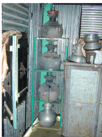
Household-based arsenic mitigation option (three- pitcher filter)
